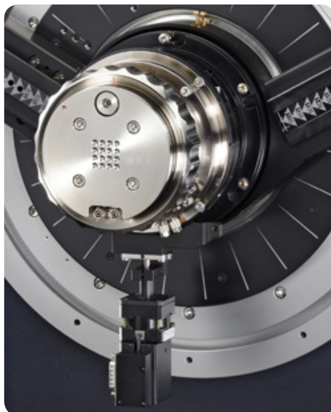
MTC-HIGHTEMP chamber with motorized height alignment stage
