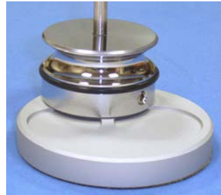
Figure 3 Loading Fixture with Specimen Figure 4 Specimen Holder on Loading Fixture
