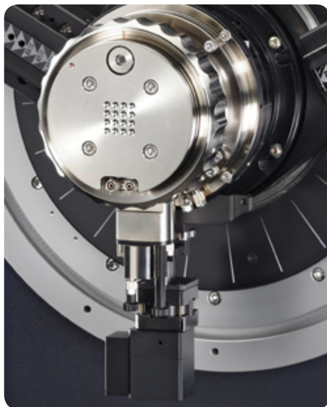
MTC-HIGHTEMP+ chamber with motorized height alignment stage
