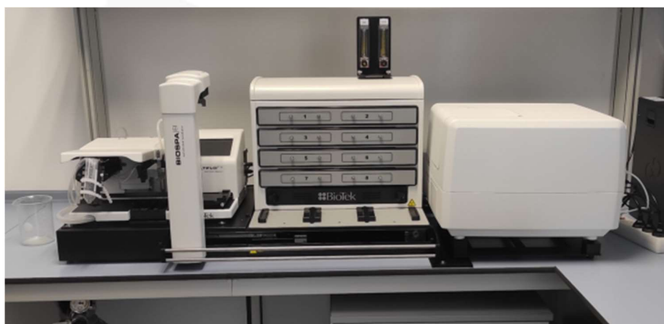
Figura 20: - Lector de placas Multimodal Synergy H1 + Multiflo FX (Bio-Tek).
