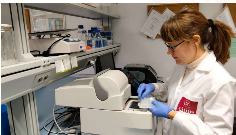
Figura 190: Termociclador PCR a tiempo real Mastercycler (Eppendorf).
