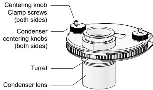
The ELWD-S Condenser supports bright-field microscopy and phase contrast microscopy. It can be used with both 100W and 30W dia pillar illuminators.
