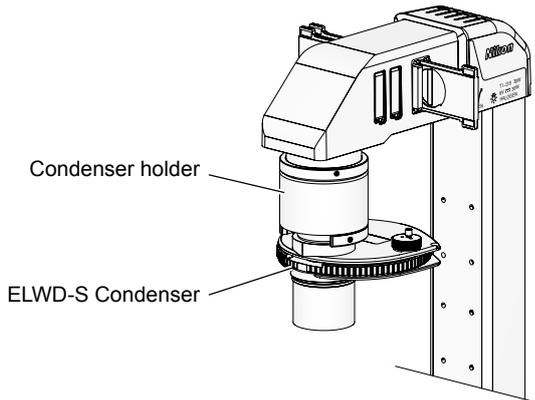
Figure 4-39 ELWD-S Condenser attachment
