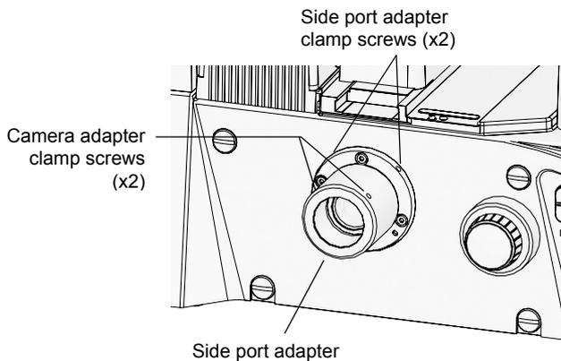
Figure 4-41 Side port adapter attachment
