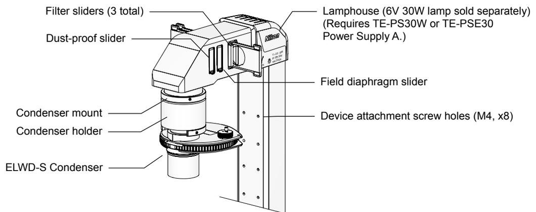
**Figure 1-22 TI-DS Dia Pillar Illuminator 30W
