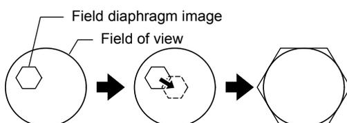
Move field diaphragm image into center of field of view. Adjust its size to match field of view.
