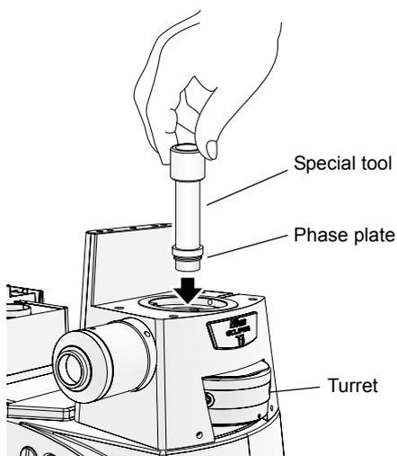
Figure 4-8 Attaching/replacing the phase plate
