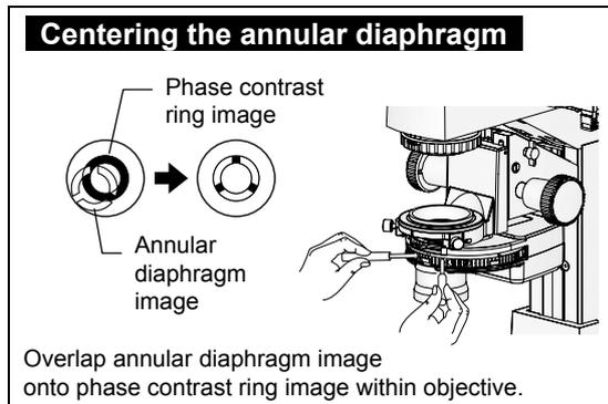
1. Move the Bertrand lens into the optical path by moving the Bertrand lens in/out lever to position "B". Adjust the focus onto the annular diaphragm image by rotating the Bertrand lens focusing knob on the right side of the eyepiece tube.
