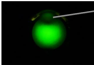
Light partially blocked in upper section of field of view.
