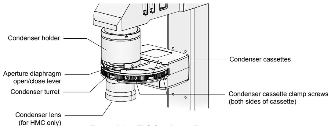
**Figure 1-24 TI-C Condenser Turret
