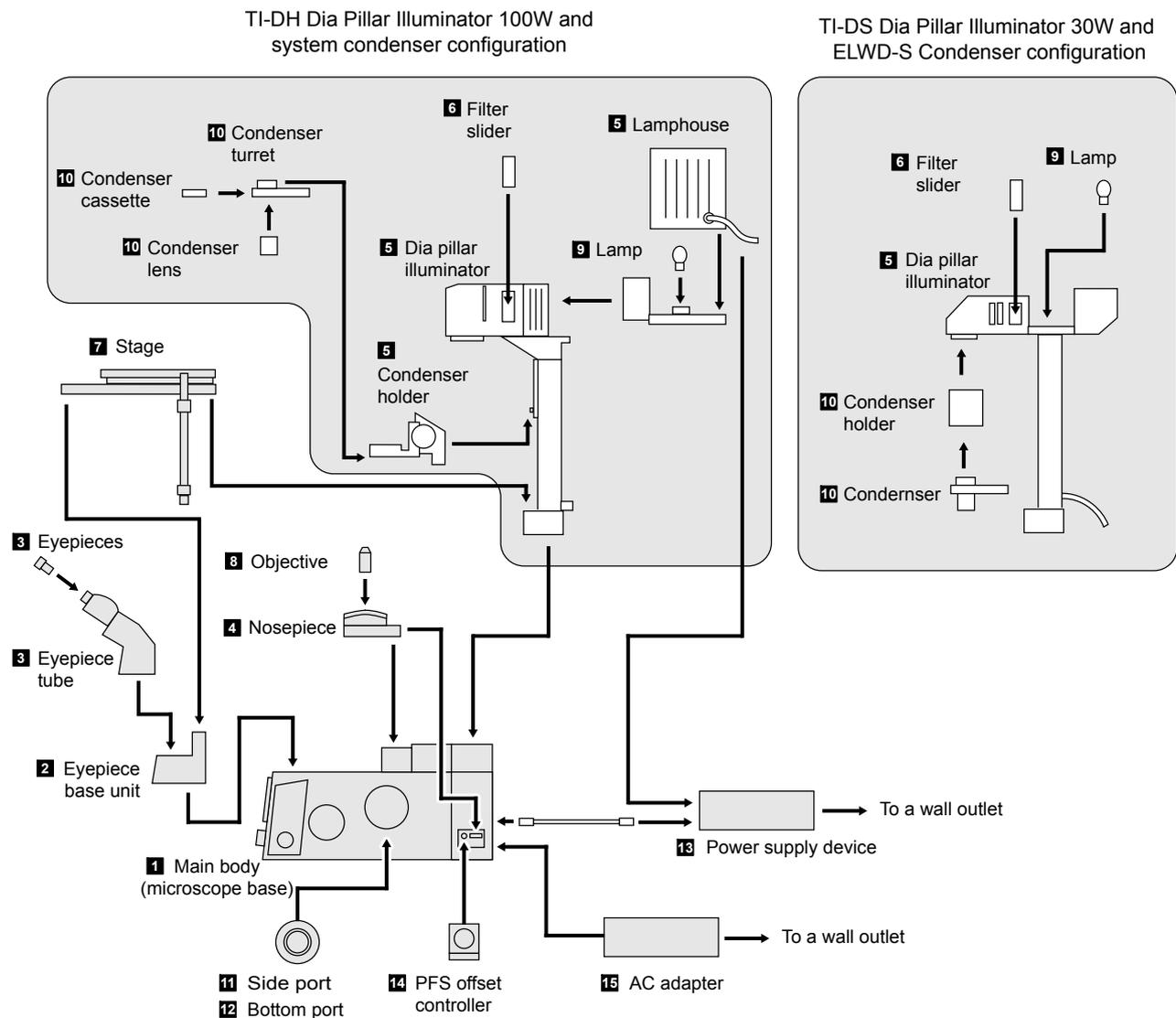
Figure 4-1 Assembly diagram
