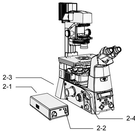
1. Set the EXTERNAL switch on the back of the power supply to "ON".
