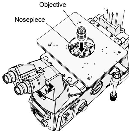
Figure 4-30 Objective attachment
