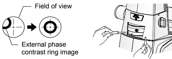
Move external phase contrast ring image into center of field of view.
