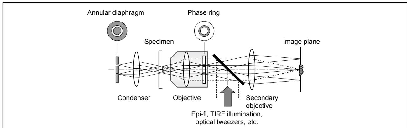
**Figure 2-2 Optical path for traditional phase contrast microscopy**
