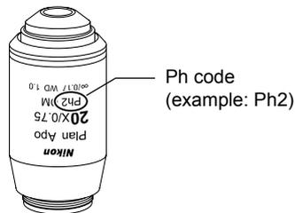
Phase contrast objectives are labeled with a “Ph code” (PhL, Ph1, Ph2, or Ph3). When performing phase contrast microscopy, use an annular diaphragm or condenser cassette that has the same Ph code as the objective, regardless of the magnification of the objective.
