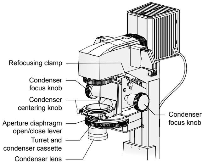
**Figure 3-19 TI-C Condenser Turret (system condenser)**
