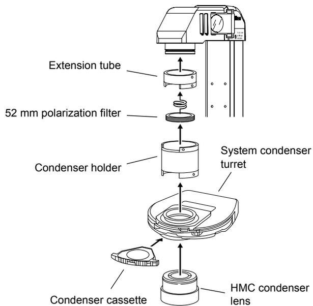
Figure 4-40 HMC Condenser attachment (system condenser)
