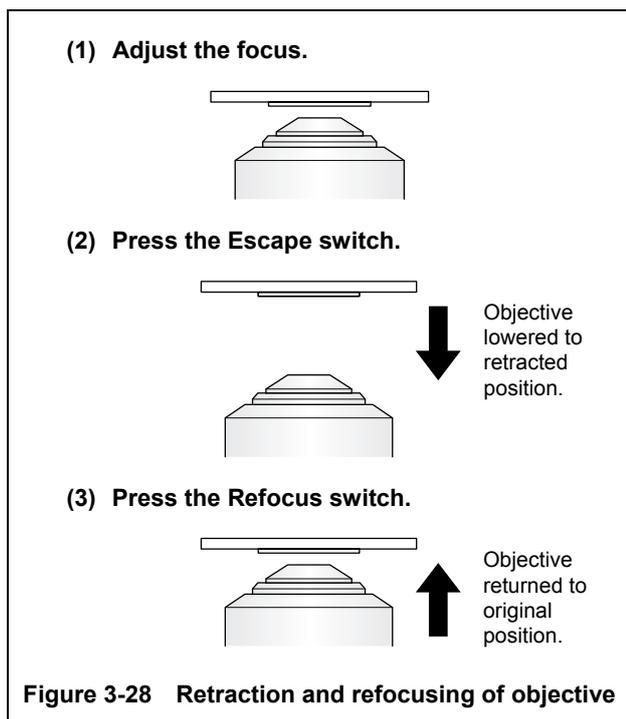
Figure 3-28 Retraction and refocusing of objective
