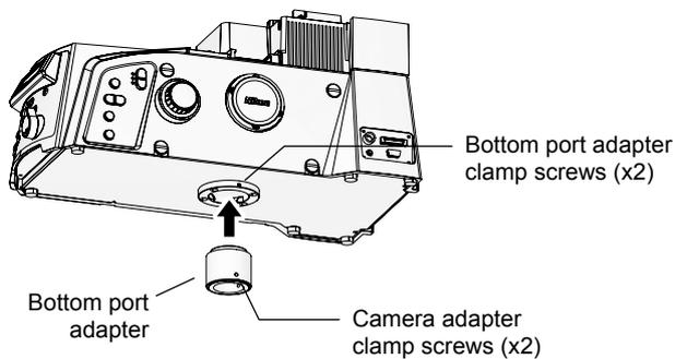
**Figure 4-42 Bottom port adapter attachment**
