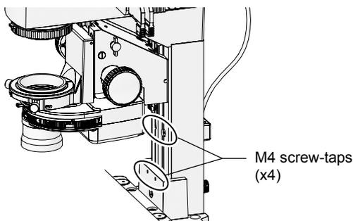
Figure 3-41 Device attachment screw holes
