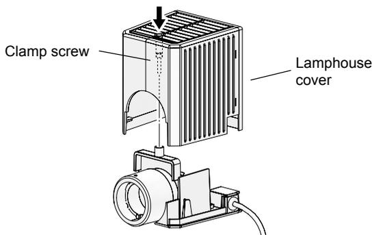
Figure 4-31 Lamphouse Cover Removal
