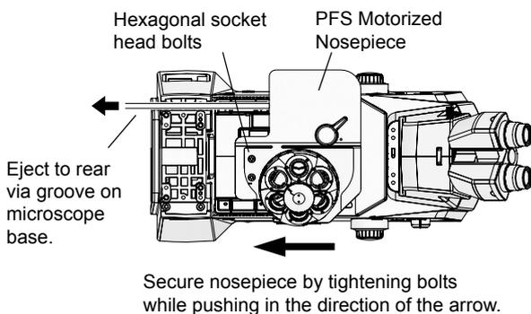
Figure 4-12 Fixing the PFS Motorized Nosepiece (top view)
