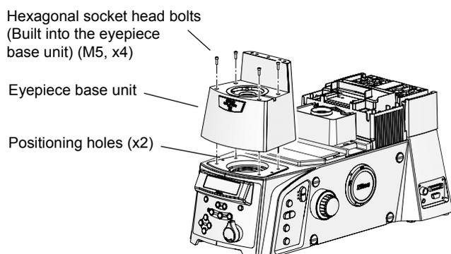
Figure 4-5 Eyepiece Base Unit attachment (TI-T-B, TI-T-BS)
