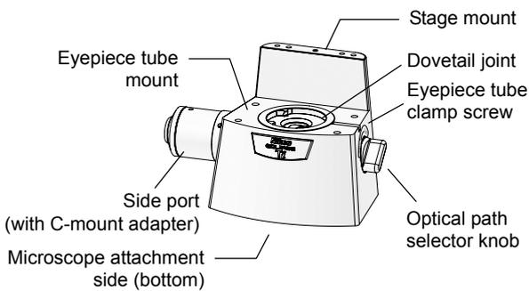
**Figure 1-11 TI-T-BS Eyepiece Base Unit (with Side Port)**
