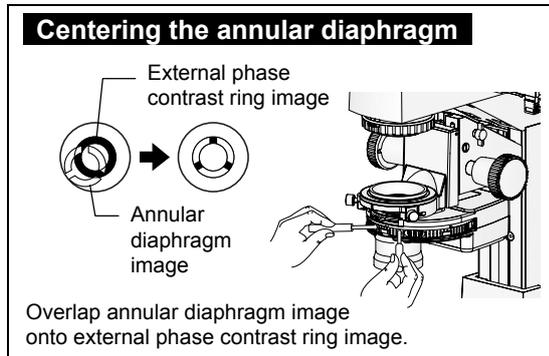
1. Rotate the condenser turret to the position for the Ph code of the external phase contrast ring in the optical path.
