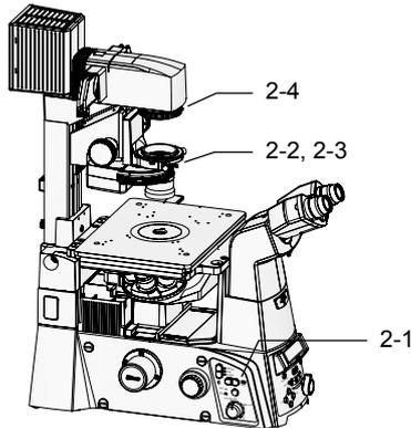
1. **Move the phase contrast objective into the optical path by pressing the Obj. switch on the left operation panel.**
