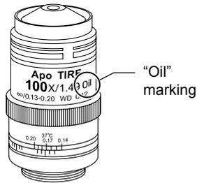
Figure 3-34 Oil immersion objective (example)
