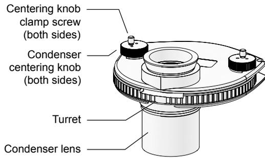
The ELWD-S Condenser supports bright-field microscopy and phase contrast microscopy. The ELWD-S Condenser can be used with both 100W and 30W pillar illuminators.
