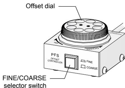
Figure 3-51 Offset adjustment
