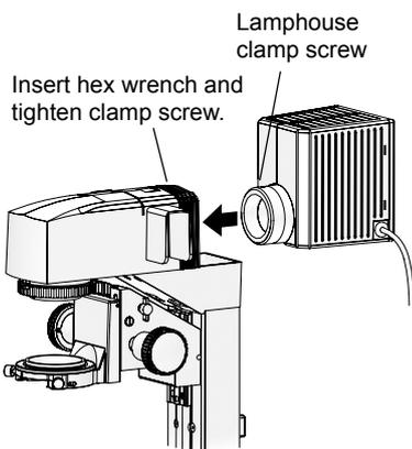
Figure 4-20 Lamphouse attachment
