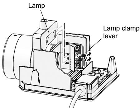
Push in lamp clamp lever to open pin hole on socket.
