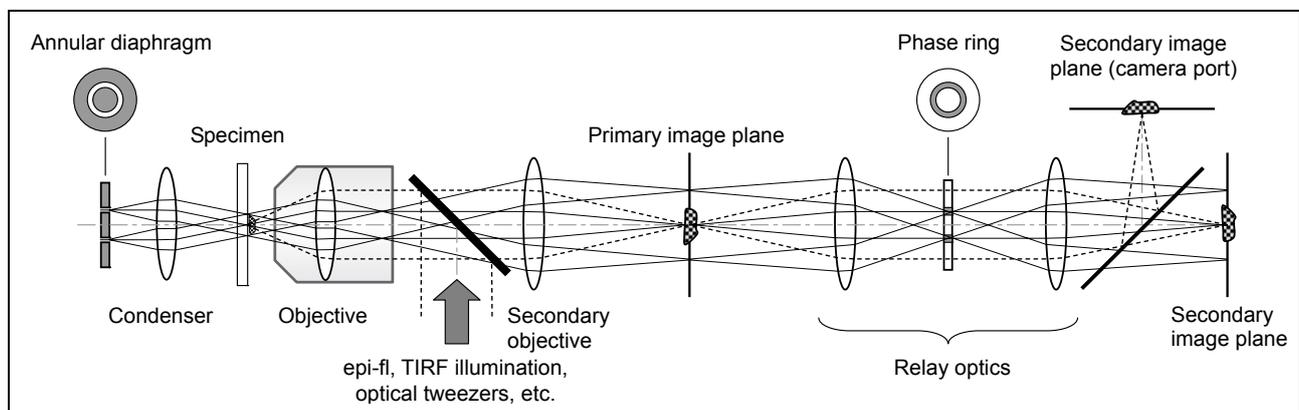
**Figure 2-3 Optical path for external phase contrast microscopy**
