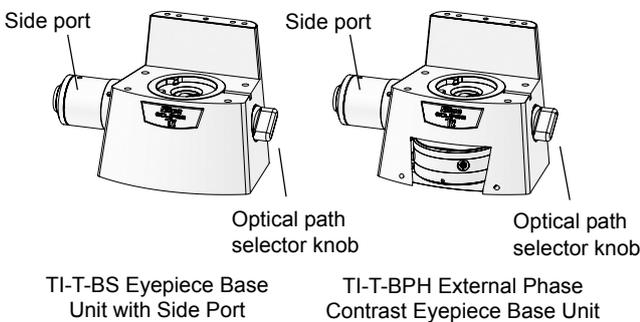
TI-T-BS Eyepiece Base Unit with Side Port
