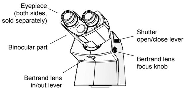
This is an eyepiece tube with a manual shutter and a Bertrand lens.
