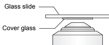
When using an objective labeled “0.17”, face the cover glass downward, and set the specimen so that the cover glass faces the objective. (The cover glass has a thickness of 0.17 mm.)
