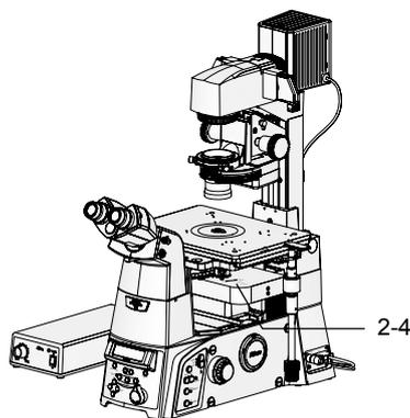
1. Move a PFS objective with the desired magnification into the optical path by pressing the Obj. switch on the left operation panel.
