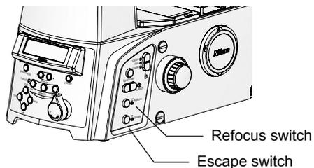
Figure 3-27 Escape switch, Refocus switch
