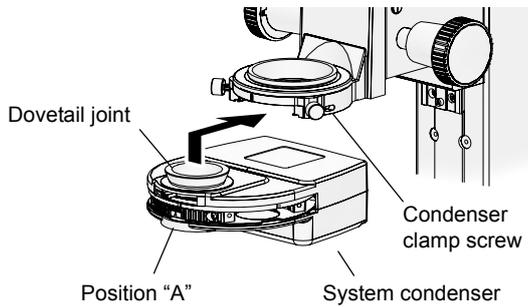
**Figure 4-36 System condenser attachment**
