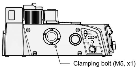
Figure 4-3 Clamping bolt
