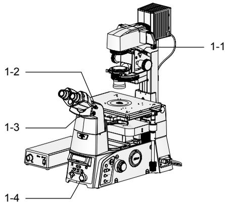
1. Release the condenser refocusing clamp on the dia pillar illuminator by rotating it counterclockwise.
