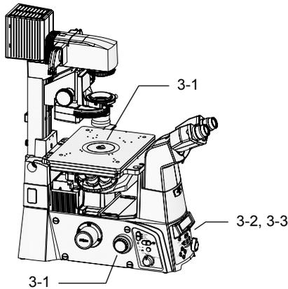
1. Move the stage to bring the observation target into the center of the field of view. Adjust the focus onto the specimen by rotating the focus knobs.
