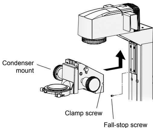
Figure 4-19 Condenser mount attachment
