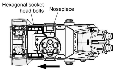
Secure nosepiece by tightening bolts while pushing in the direction of the arrow.
