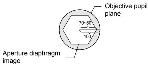
Adjust the size of the aperture diaphragm image to 70-80% the size of the objective pupil plane.
