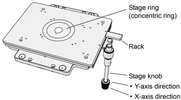
Figure 1-18 Rectangular Mechanical Stage
