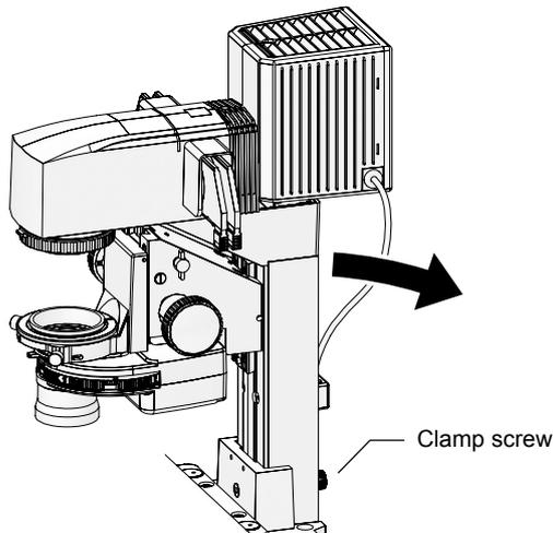
Figure 3-40 Pillar inclination
