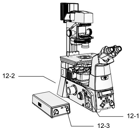
1. Turn off the dia illumination by pressing the dia illumination lamp ON/OFF switch on the left side of the microscope.
