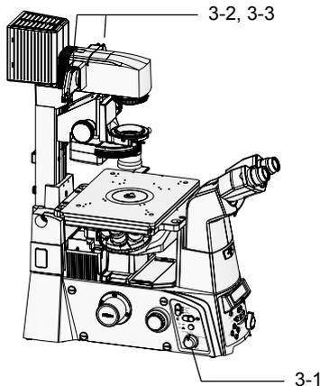
1. Rotate the brightness control knob on the left side of the microscope to the “12V100W” position.
