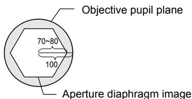
Adjust the size of the aperture diaphragm image to 70-80% the size of the objective pupil plane.
