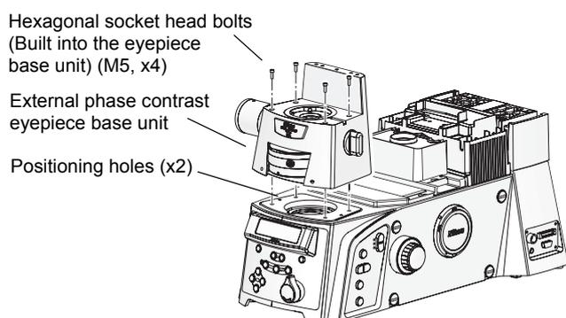
Figure 4-6 External phase contrast eyepiece base unit attachment
