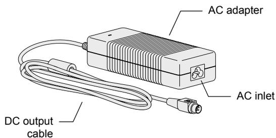
**Figure 4-46 AC adapter**
