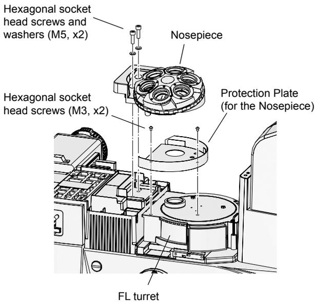
1. Using a 2 mm hex screwdriver, remove two of four M3 hex socket head screws from the top of the filter turret (TI-FLC, TI-FLC-E, or TI-FLC-E/HQ), as shown in the figure at left.
