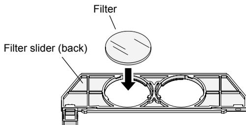
Although the filter slider for the 30W dia-illuminator has a different shape, the method for securing the filters is the same.
