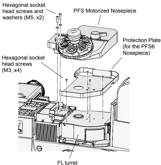
**Figure 4-16 Protection Plate (for the PFS6 Nosepiece) attachment**
