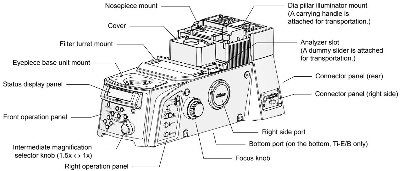
**Figure 1-3 Microscope base**
