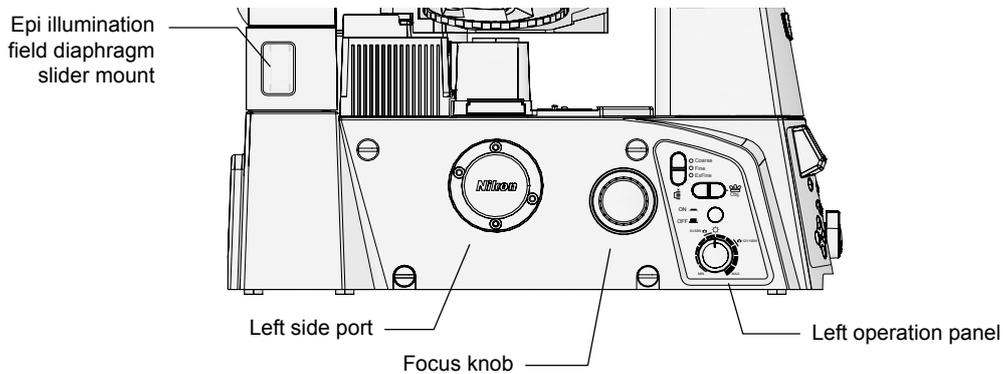
**Figure 1-4 Microscope base (left view)**
