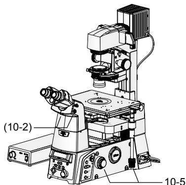
1. Move an objective with the desired magnification into the optical path by pressing the Obj. switch.
