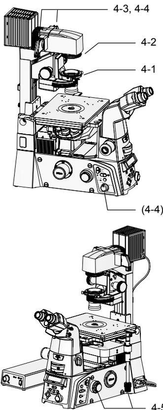
1. Fully open the aperture diaphragm of the condenser.
