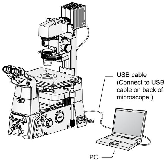
**Figure 4-48** Connecting microscope and PC (example)
