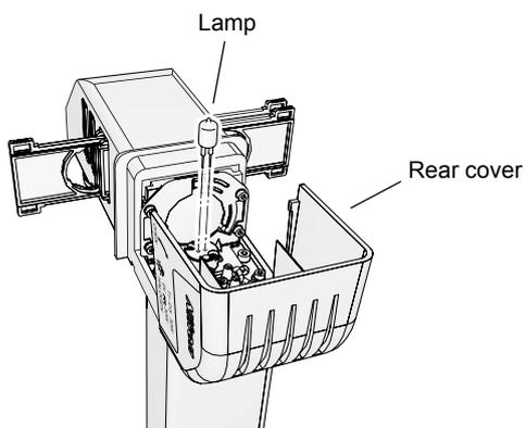
Figure 4-34 Replacing lamps
