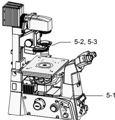
1. Move a phase contrast objective with the desired magnification into the optical path by pressing the Obj. switch.
