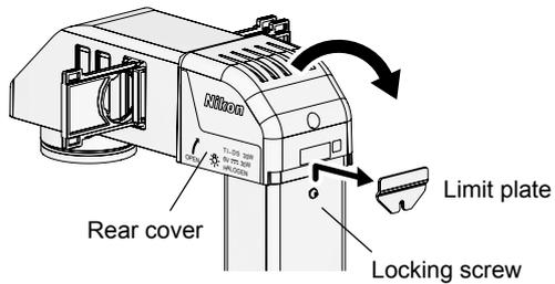
Figure 4-33 Rear cover of the lamphouse
