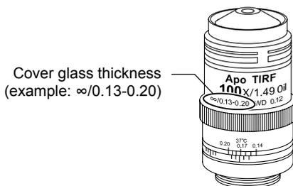
Objectives are labeled with the supported cover glass thickness. For example, “∞/0.17” indicates a cover glass thickness of 0.17 mm.
