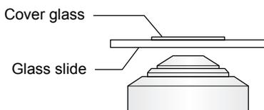
When using an objective labeled “1.2”, face the cover glass upward, and set the specimen so that the glass slide faces the objective. (The glass slide has a thickness of 1.2 mm.)
