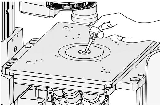
Figure 3-35 Applying oil immersion
