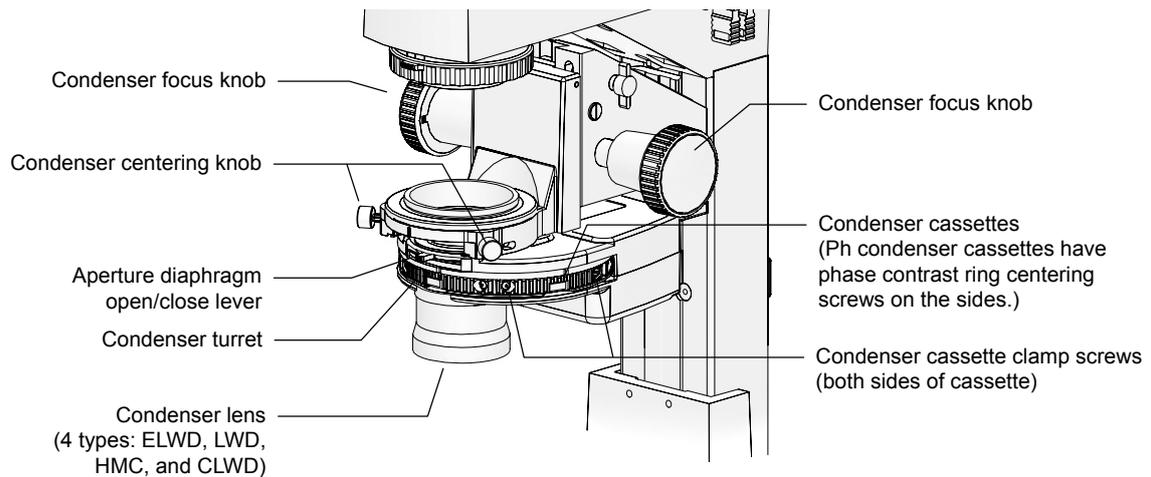
**Figure 1-23 TI-C Condenser Turret
