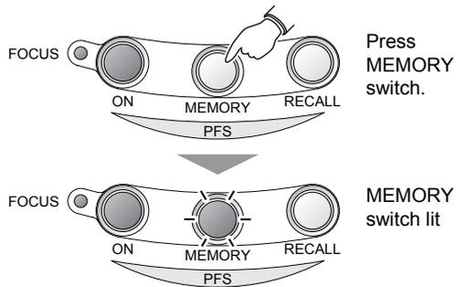
Figure 3-52 Registering the offset
