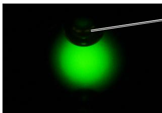
Air bubble recognized in upper section of field of view.
