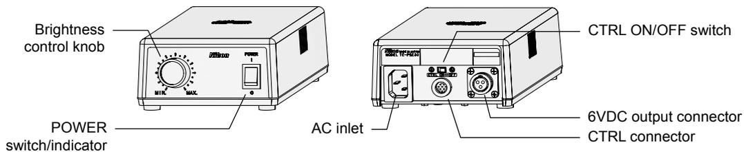
Figure 1-27 TE-PS30W, TE-PSE30 Power Supply A
