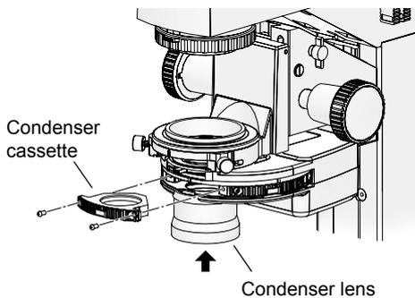
**Figure 4-37 Condenser cassette and condenser lens attachment**
