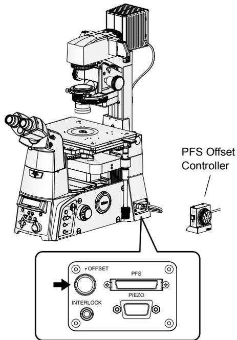
When using the PFS Motorized Nosepiece, connect the PFS Offset Controller to the Ti-E or Ti-E/B microscope body.
