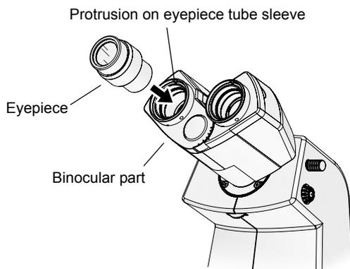
Figure 4-10 Eyepiece attachment
