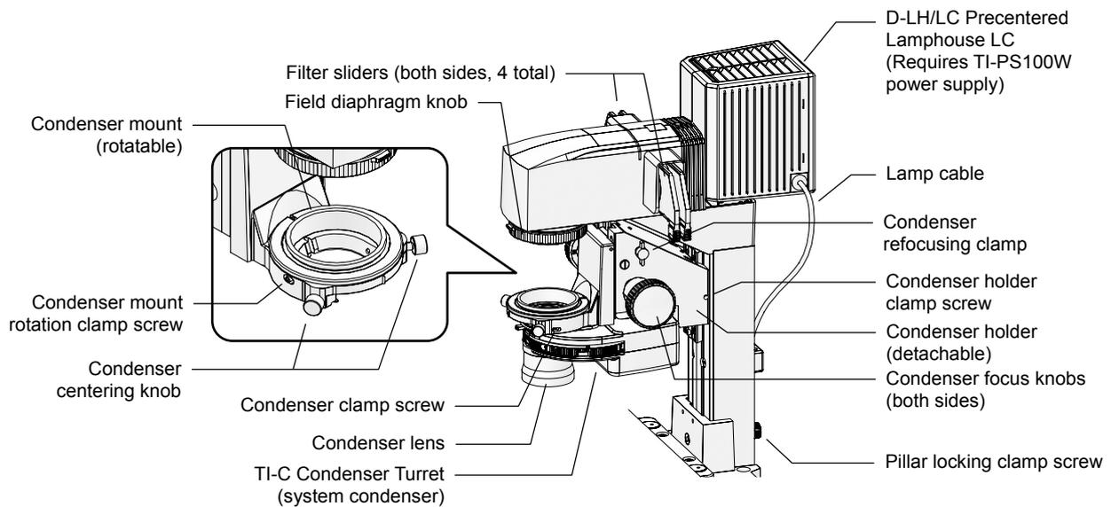
**Figure 1-21 TI-DH Dia Pillar Illuminator 100W
