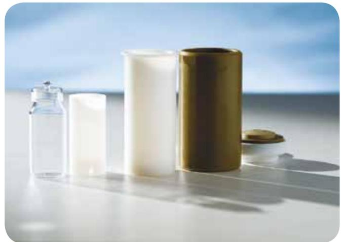
A large selection of high purity quartz and TFM inserts is available for all Milestone pressure vessels, for smaller sample amounts or to minimize the dilution factor of the analytical solution.
