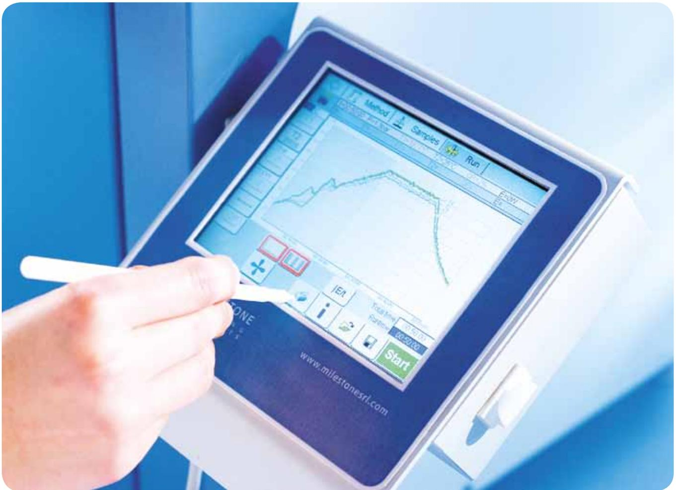
The ETHOS One is operated via a compact control terminal with easy-to-read, bright, full-color, touch-screen display.
