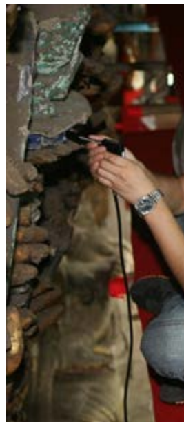
Direct contact measurement of pigments on a statue/wall.
