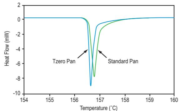
The utility of the Tzero hermetic pan is shown here. In this example, DSC results for casein are shown using both a hermetic pan and a standard pan. Casein contains a significant amount of adsorbed moisture, which is evolved when heating in a standard pan. The resultant data only exhibits the large evaporation endotherm. However, when analyzed in a Tzero hermetic pan, the volatilization is suppressed, and the glass transition of the casein is clearly identified.
