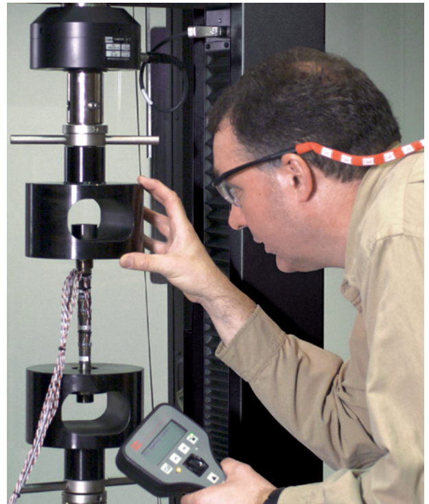
Load Frame Alignment
