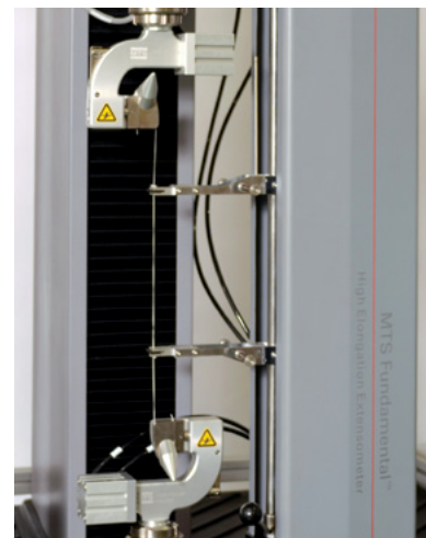
High Elongation Extensometer
