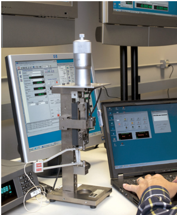
Extensometer Calibration
