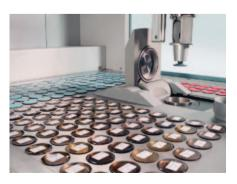
changer is available which can accomodate up to 209 uncupped samples of 32 mm or 140 uncupped samples of 40 mm diameter.
