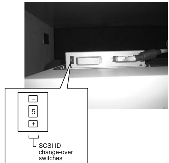
Fig. 2.13 SCSI ID Change-Over Switches
