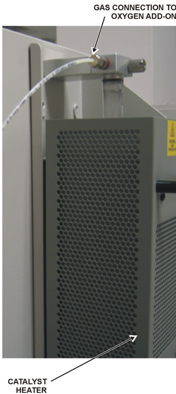
Figure 3-21 Catalyst Heater Gas Connection
