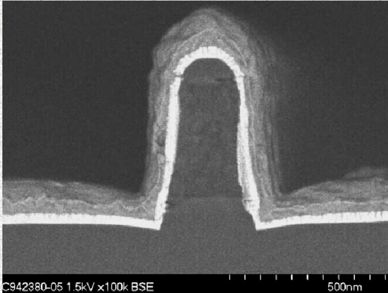
Ta barrier under Cu Seed
